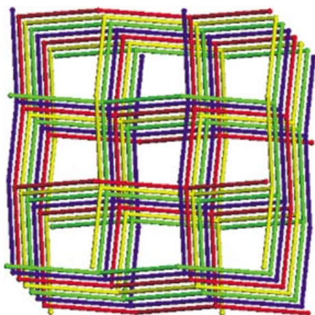
Figure 5. Schematic view of the cluster coordination polymer 1 . The cationic and anionic cluster coordination polymers are shown in blue/yellow and red/green, respectively. (The blue/yellow node and rod represent the cluster cation and the double 4,4'-bipy ligand, respectively; the red/green node and rod represent the cluster anion and the single 4,4'-bipy ligand, respectively.)
